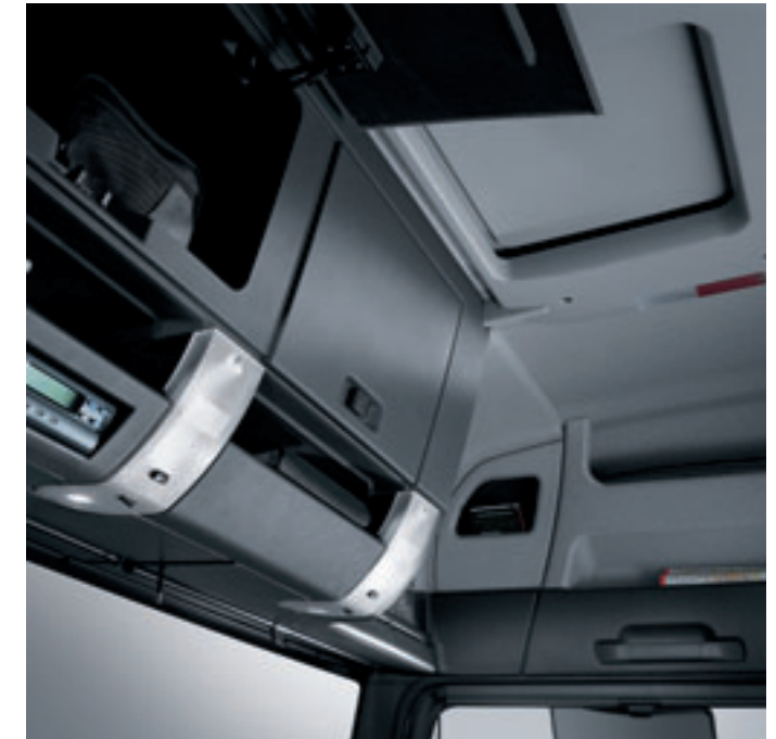
Roof storage compartments above the front windscreen and electrical roof hatch in the LX driver's cab
