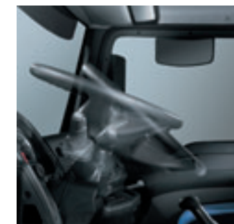
Steering wheel steplessly adjustable in height and rake by foot-operated button
