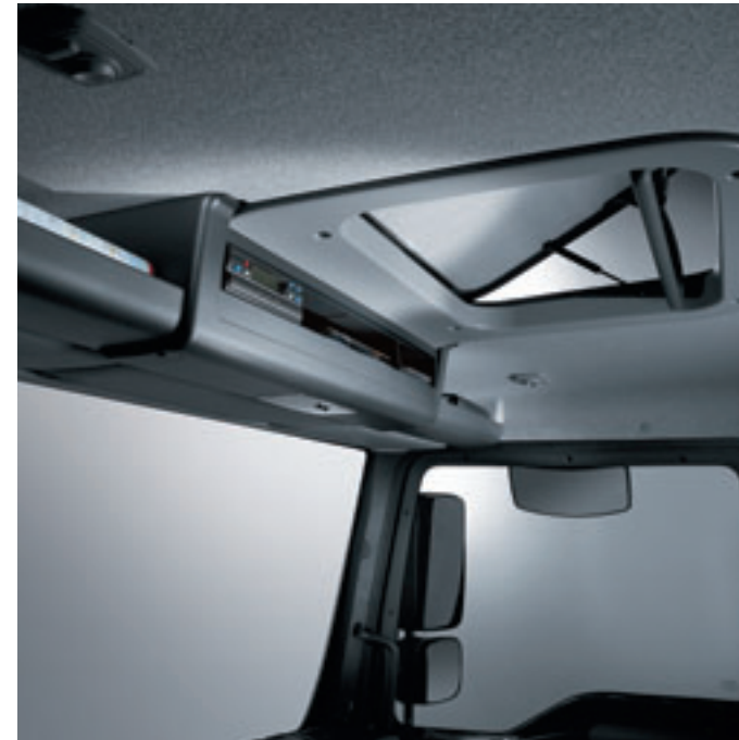
Storage compartment above the windscreen and roof hatch in the C cab
